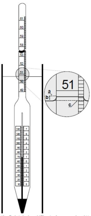
Note: To obtain the observed API gravity of an opaque crude, read (a)  $50.8^{\circ}$ API, the top of the meniscus; and then subtract (b)  $0.1^{\circ}$ API, the height of the meniscus to find (c)  $50.7^{\circ}$ API, the actual liquid surface level.
